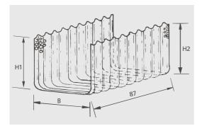
Corners can easily be made by the client by cutting and tying with wire on site. Photos 1, 3 and 4 show a building section with shuttering partially filled with concrete, soil or still freestanding.
